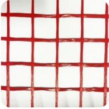
**OLY MESH GLASS 250** is a preformed structural fiberglass mesh AR (alkaline resistant, with at least 17% zirconium) for structural reinforcement and consolidation of masonry, floors, screeds, vaults, concrete and flooring. Suitable for anti-shelling of floors and for anti-overturning of primary and secondary partitions.
