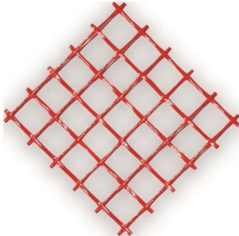
**OLY MESH GLASS 150** is a pre-formed structural mesh in AR glass fiber (alkaline resistant, with at least 17% zirconium) woven with a leno and primed with PVA suitable for structural reinforcement and consolidation of walls, floors, screeds, vaults, concrete and flooring . Suitable for the anti-shattering of floors and for the anti-tilting of primary and secondary partitions.
