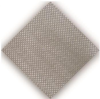
**OLY TEX GLASS 1140 QUADRI-AX HR** is a quadriaxial balanced glass fiber fabric with a weight of 1140 g/m<sup>2</sup> with high mechanical resistance specific for structural consolidation interventions of masonry, wood and in some cases in reinforced concrete.
