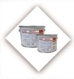
The two-component epoxy system OLY RESIN 10 HTG is a thixotropic epoxy putty, CE-marked according to EN 1504-4 as structural bonding, solvent-free, specially designed for bonding FRP foils, impregnation of steel fabrics for SRP systems, bonding of metal plates and regularisation of substrates. The resin part is white while the hardener part is black. It can be applied by trowel on surfaces that have been previously prepared and where applicable suitably treated with OLY RESIN BASE DB.
